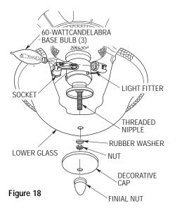
□ 11. Your ceiling fan is now installed and wired to be controlled by your remote control system.
